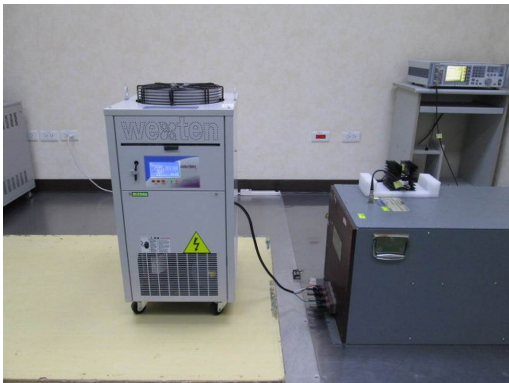
Picture 17: Test setup for Conducted Susceptibility, CWIDA04PTS (AC 400V)
