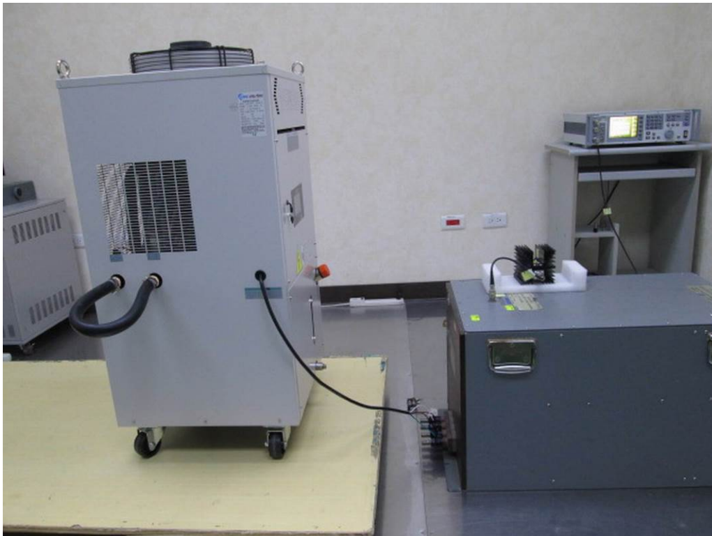
Picture 35: Test setup for Conducted Susceptibility, CWIDA12PTS (AC 400V)
