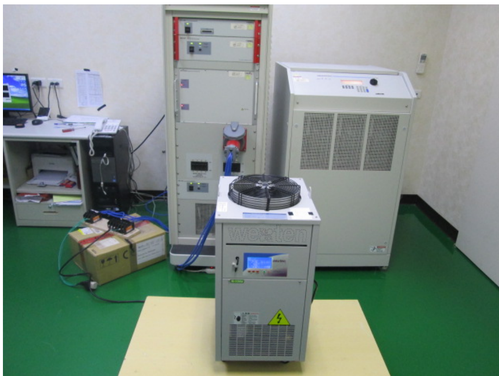
Picture 12: Test setup for Harmonics/Flickers, CWIDA04PTS (AC 400V)
