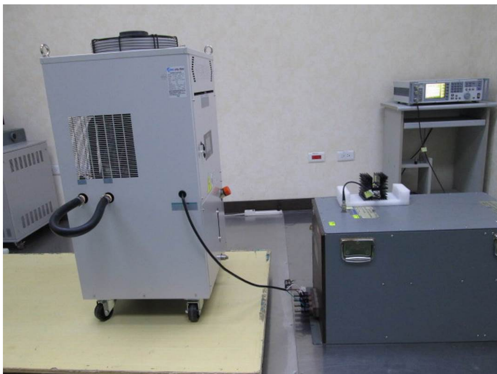
Picture 26: Test setup for Conducted Susceptibility, CWIDA12PTS (AC 230V)
