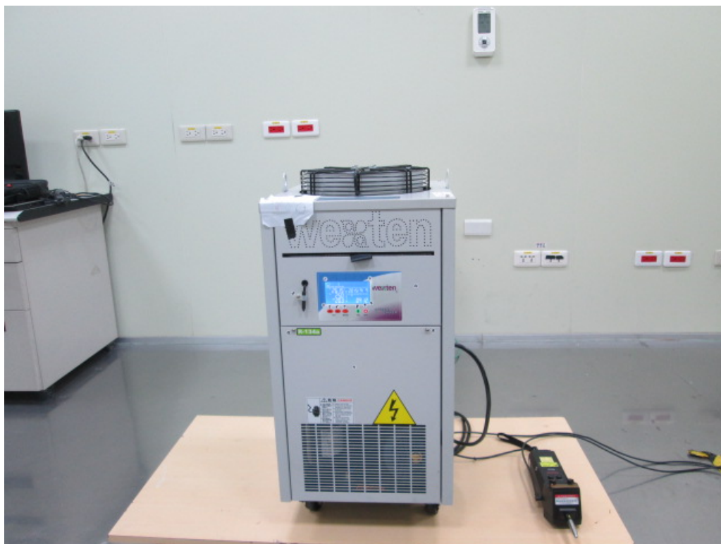
Picture 13: Test setup for Electrostatic Discharge, CWIDA04PTS (AC 400V)
