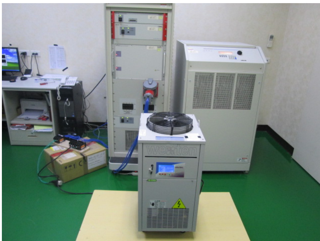
Picture 18: Test setup for Voltage Dips and Interruption, CWIDA04PTS (AC 400V)
