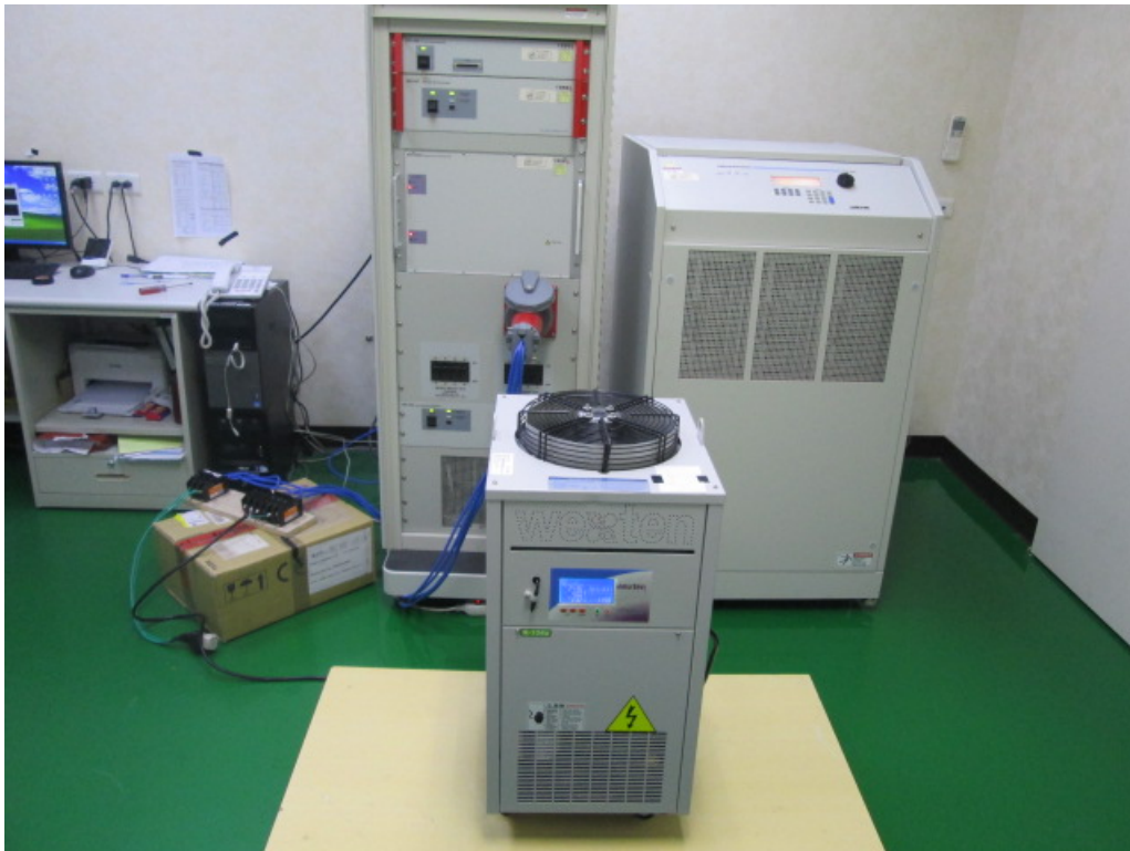
Picture 3: Test setup for Harmonics/Flickers, CWIDA04PTS (AC 230V)
