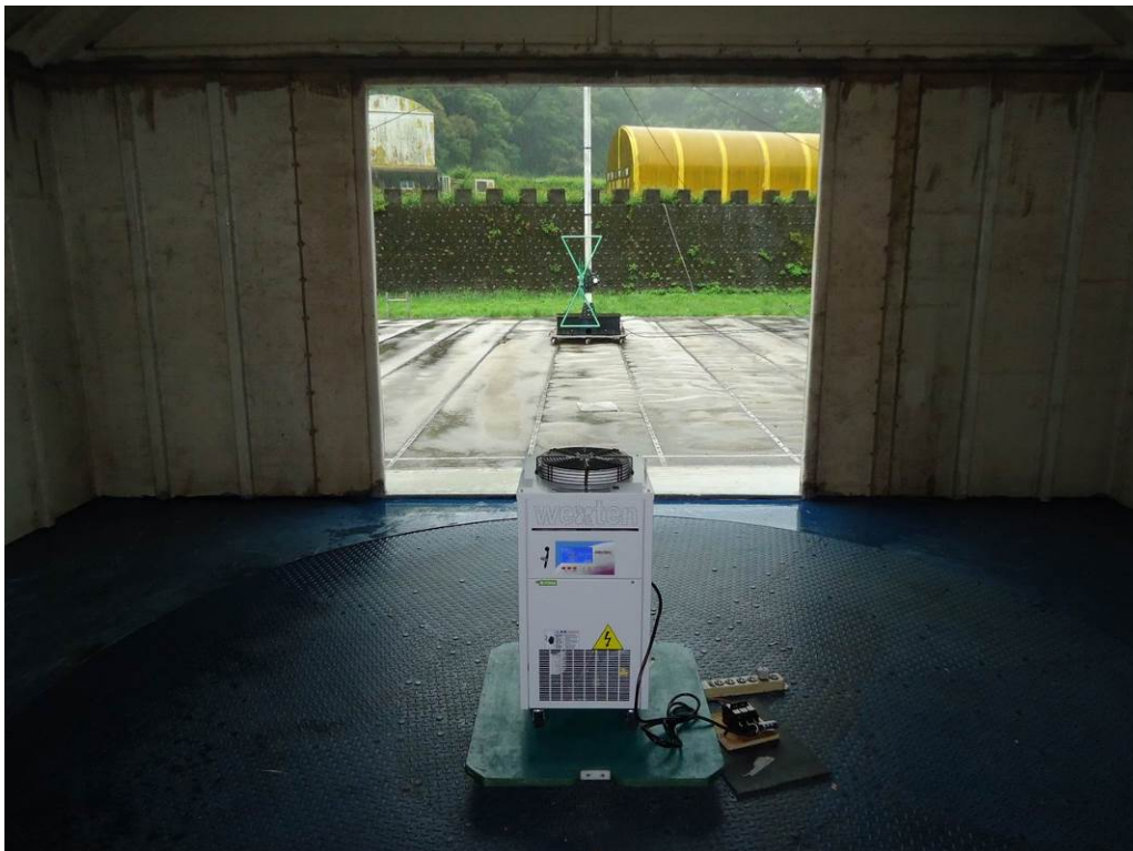
Picture 2: Test setup for Radiated Emission, CWIDA04PTS (AC 230V)
