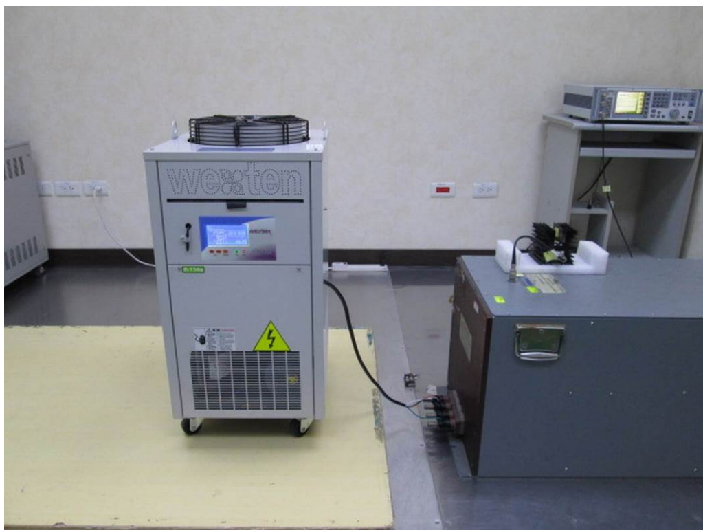
Picture 8: Test setup for Conducted Susceptibility, CWIDA04PTS (AC 230V)
