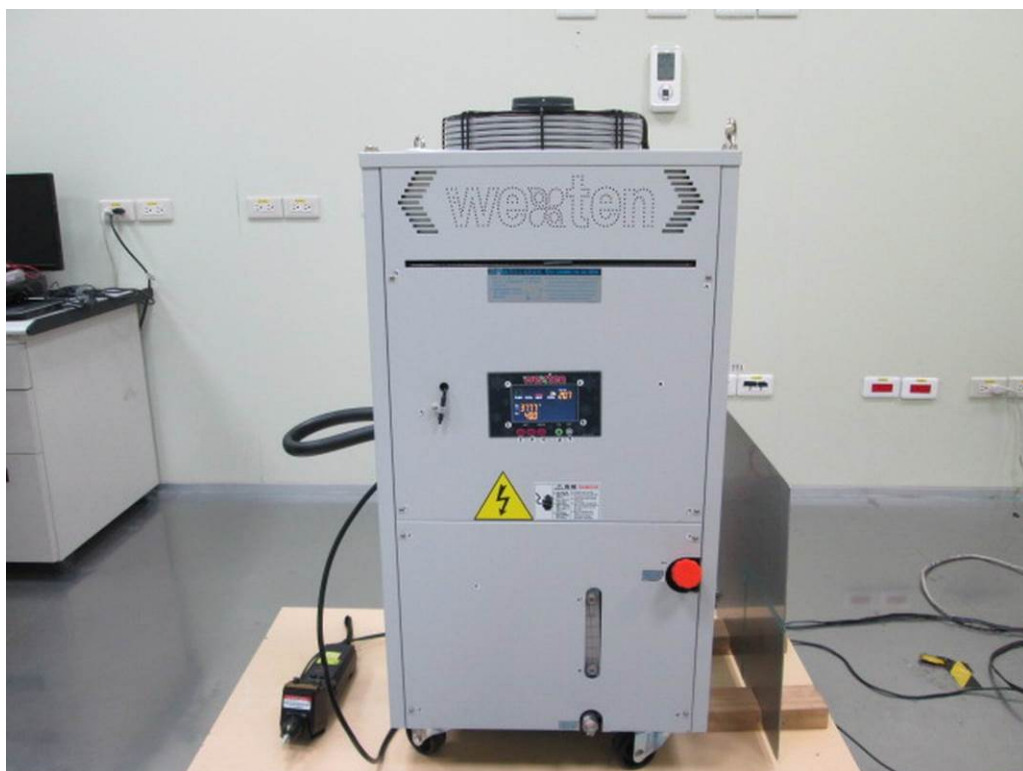
Picture 22: Test setup for Electrostatic Discharge, CWIDA12PTS (AC 230V)
