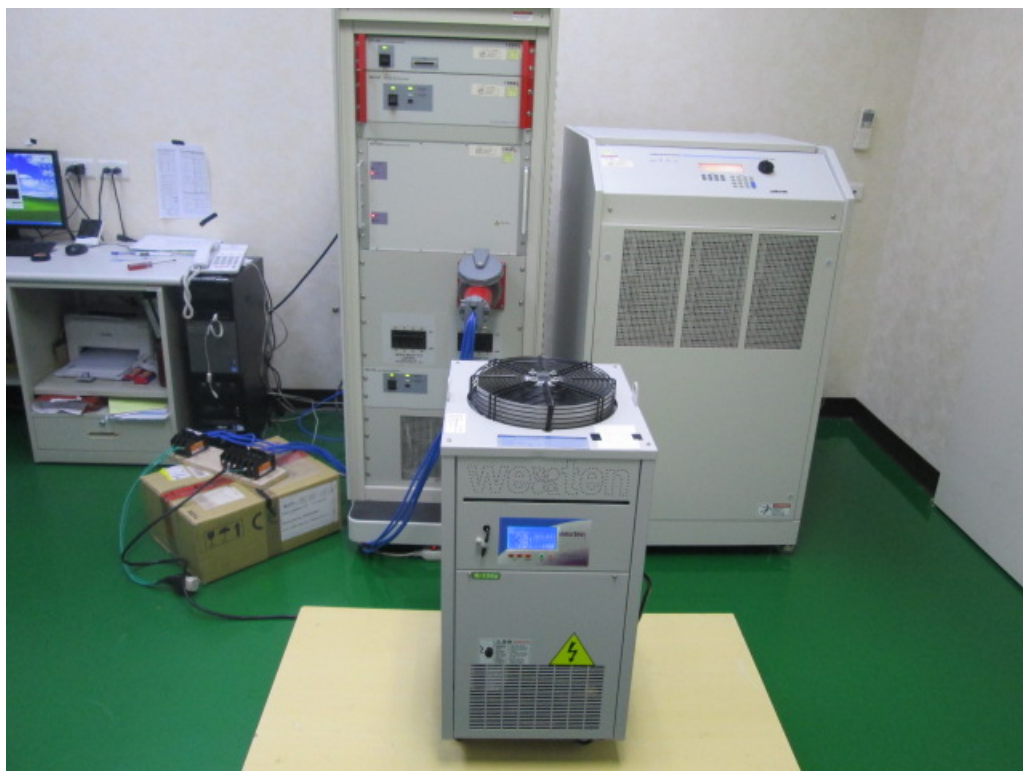
Picture 9: Test setup for Voltage Dips and Interruption, CWIDA04PTS (AC 230V)
