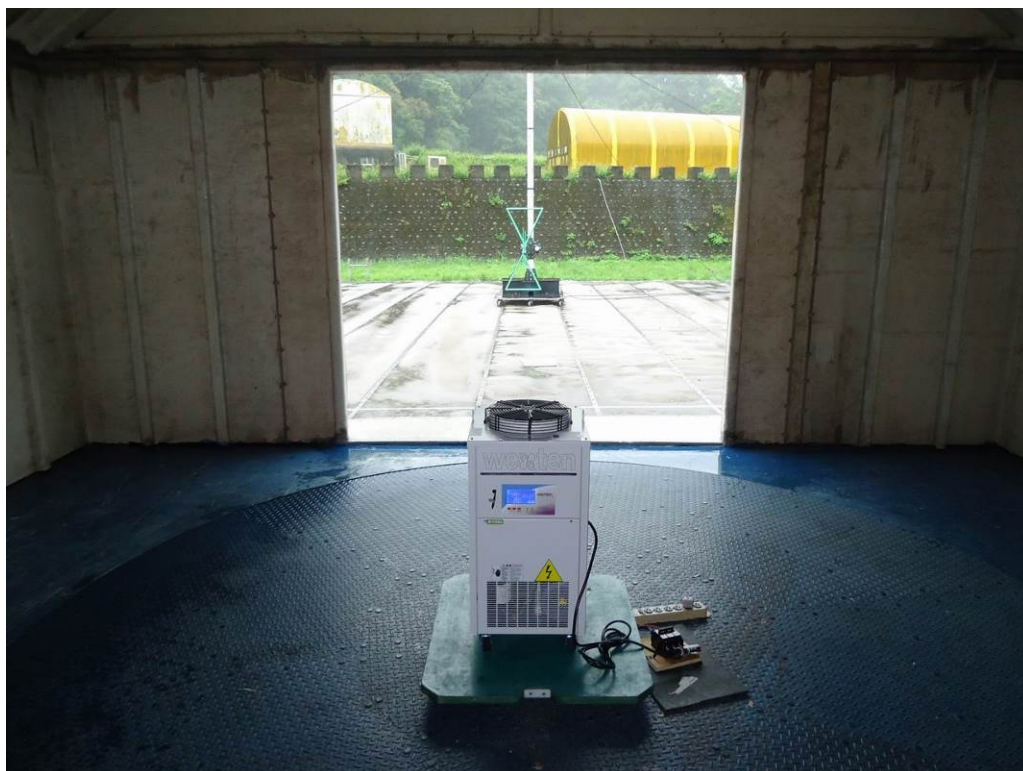
Picture 11: Test setup for Radiated Emission, CWIDA04PTS (AC 400V)
