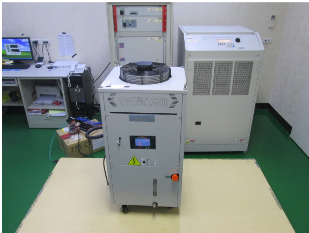
Picture 27: Test setup for Voltage Dips and Interruption, CWIDA12PTS (AC 230V)
