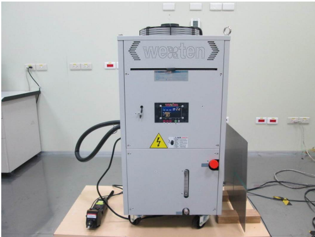
Picture 4: Test setup for Electrostatic Discharge, CWIDA04PTS (AC 230V)
