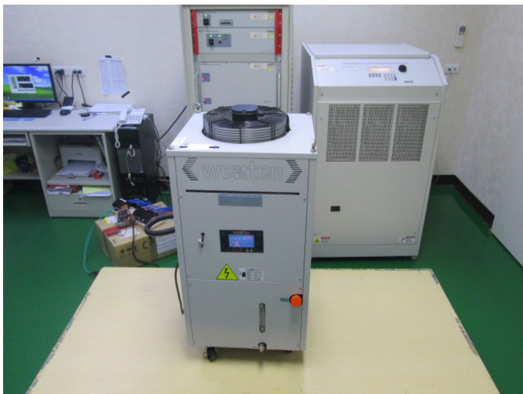
Picture 30: Test setup for Harmonics/Flickers, CWIDA12PTS (AC 400V)
